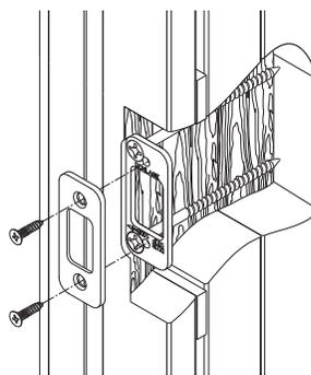
Strike reinforcement plate with 3" screws provides maximum resistance to kick-in attacks.
